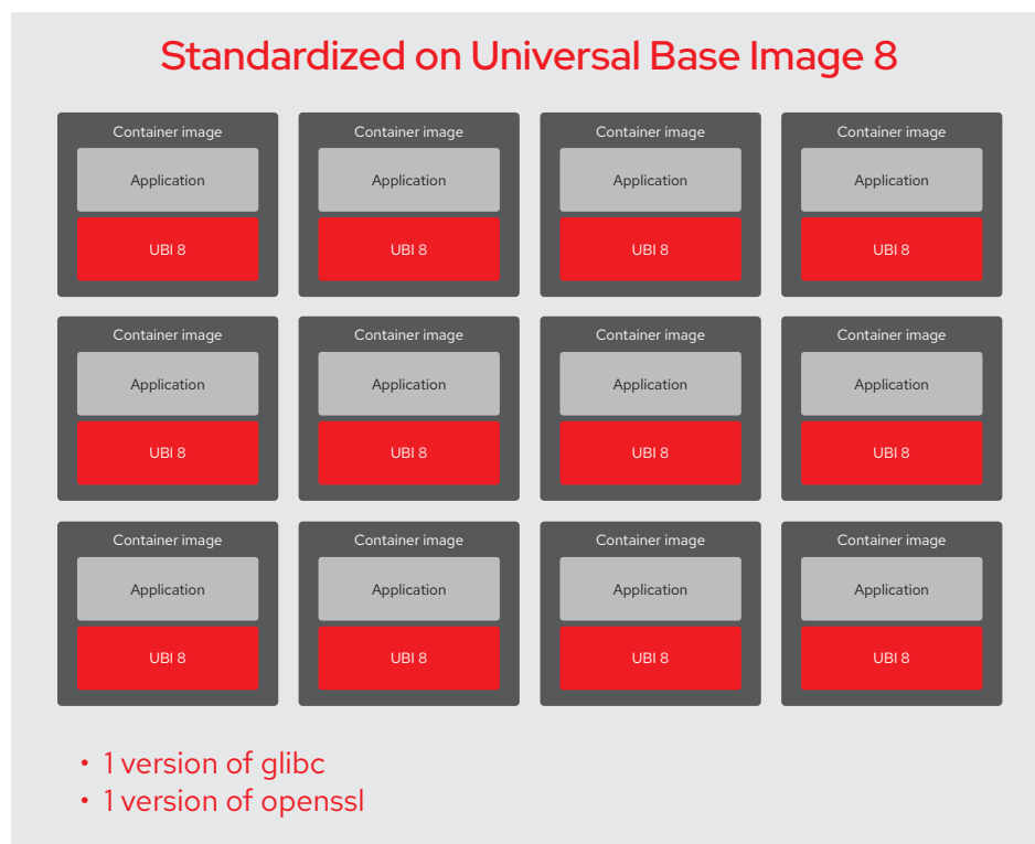
Figure 4. Standardizing on a container base image to control software versions
