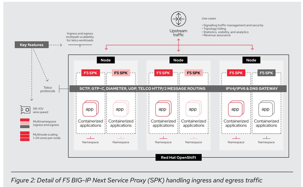
Figure 2: Detail of F5 BIG-IP Next Service Proxy (SPK) handling ingress and egress traffic
